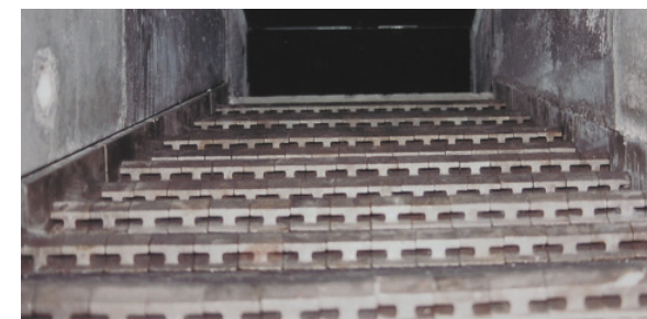
Flat moving grate FSB - hydraulically driven (two independently moving sub-grates available for boilers with a nominal capacity of 850 kW / 2.9 MBTU/h and larger)
