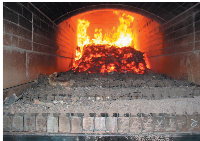
Figure 2: MAWERA flat moving grate in operation
