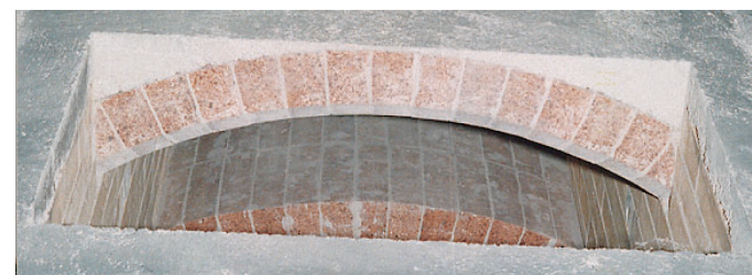
Figure 4: Refractory lining on top of the vaulted MAWERA combustion chamber
