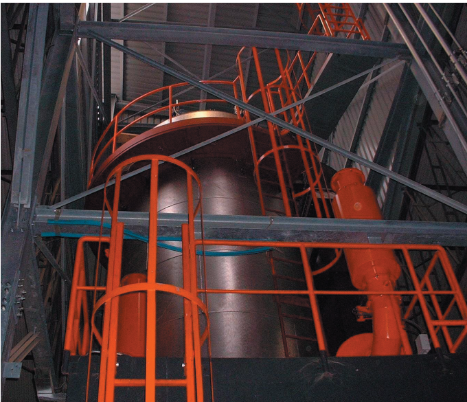
Figure 10: Thermal oil boiler on top of a 20 MBTU/h (6 MW) MAWERA firebox boiler model FSR
