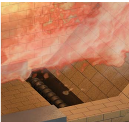
Optimal automatic ash removal via water-cooled screw conveyor
