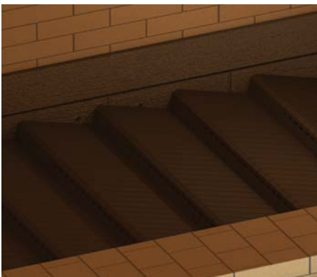
Hydraulically driven flat moving grate
